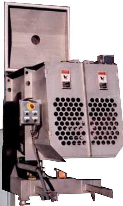
weight of the hydrated rice is more likely to crush the soft kernels during agitation and discharge. The Steam-Therm is specially designed with a short tub length, large diameter, and an extra large discharge door. The agitator paddles are large to push the rice through the oversized door with fewer revolutions and minimum pressure on the fragile rice kernels.
