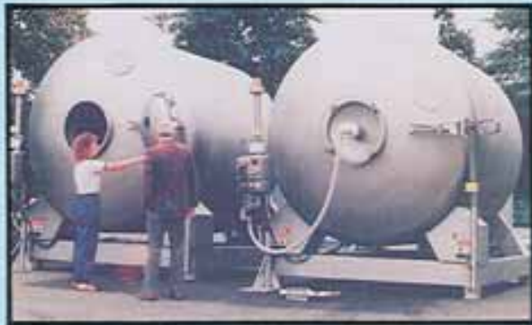
TWO 10,000 LB. CAPACITY PRODUCTION VACUUM TUMBLER-MIXERS.
