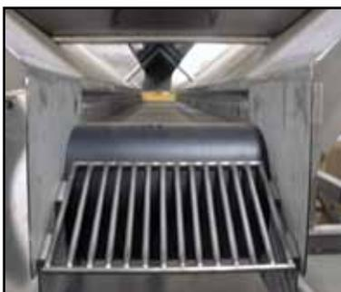
Discharge end of a belt discharge bulk bin.
