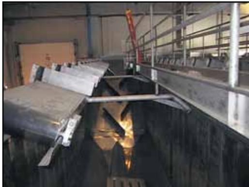
Slanted inlet end, lowerator, and tilted bin fill conveyor are exclusive features of Vanmark bins.
